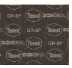
Soft sealing material reinforced with pegged steel core offers excellent thermal and stress resistance combined with very good adaptability to flange irregularities. Due to metal reinforcement it shows very good resistance to "blow-out".
